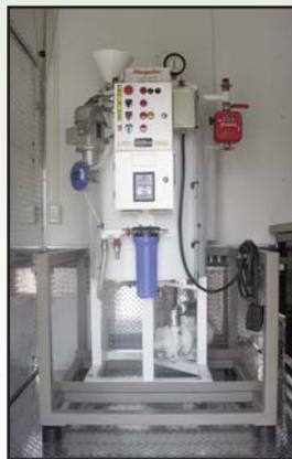
The Hampden **Model H-BIO-100** Bio Diesel Demonstrator is ideal for educational purposes, using the same protocol and with the same quality construction as the large scale units. The rugged design, capacity and ease of use make this unit ideal for teaching and experimentation.
