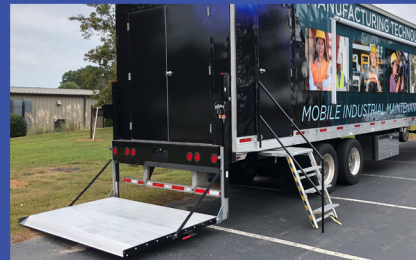
Multiple access points including two side doors and large double doors with power lift at the rear.
