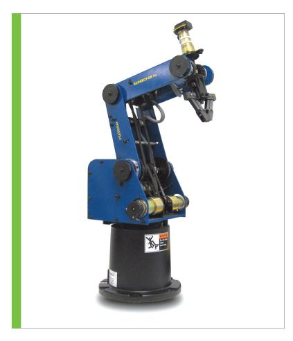
The ScorBot ER-4U robot is a versatile and reliable 5-axis robotic arm system for educational use. The ScorBot ER-4U robot arm can be mounted on a tabletop, pedestal, or linear slidebase.
